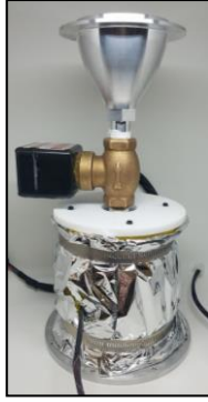
Figure 4. Propulsion system, unintegrated.
